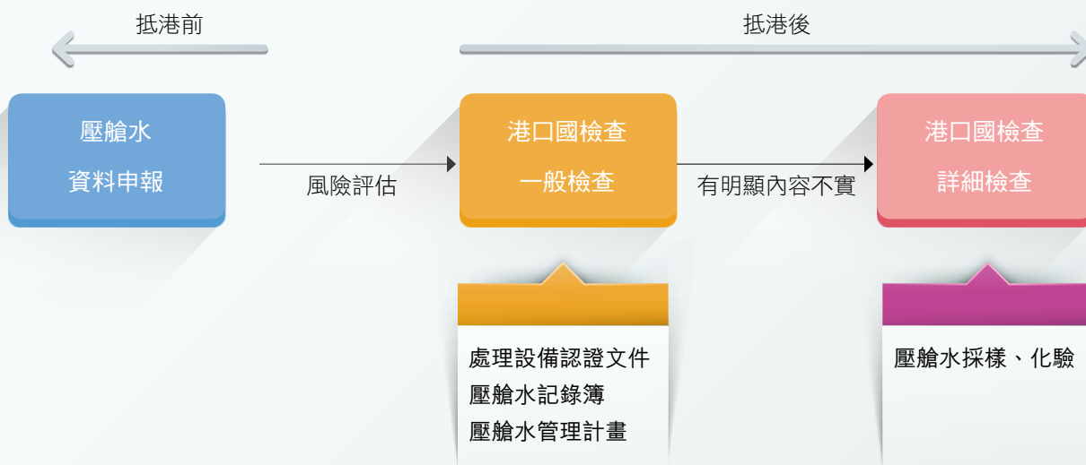
Figure 4-24 Flow Chart of Ballast Water Management in the Ballast Water Management Convention
