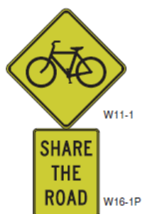
Figure 4-1. "Share the Road" Sign Assembly
