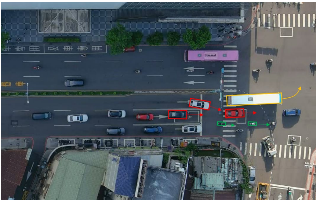
Note: Identifying Cars (Red) and Motorcycles (Green) in Upstream Traffic of the Left-Turn Lane Figure 3: Poor “Left-Turn Lane Configuration” Causing Left-Turn Waiting Vehicles to Disrupt Straight-Moving Traffic
