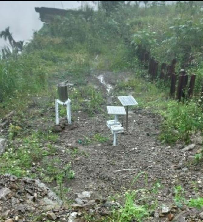
A photograph showing a rain gauge station in a field. The rain gauge is a white cylindrical device mounted on a white metal stand. To its right, there is a solar panel mounted on a white metal frame. The ground is a mix of dirt and small rocks, and there is some green vegetation in the background. |
