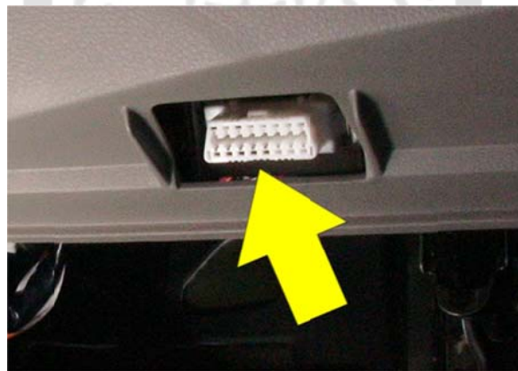
Figure 1.A connector of the on-board diagnostic(OBD)device.
