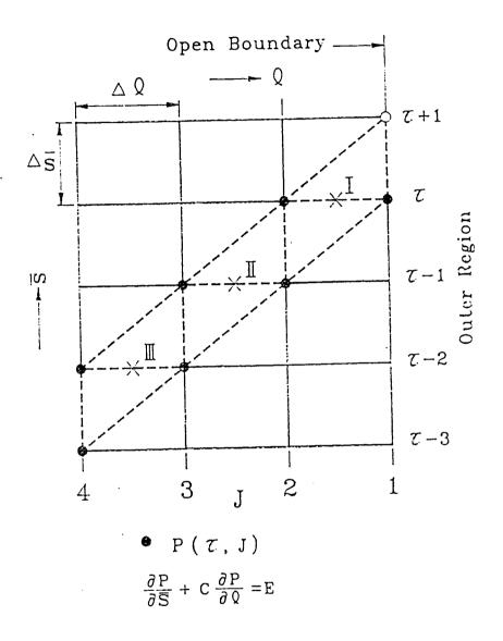
Fig. 2 Discretization on the open boundaries
