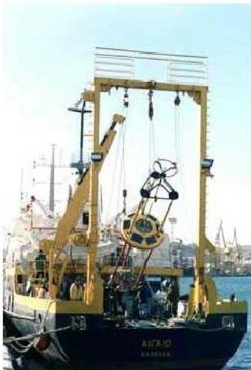
The SEAWATCH buoy on board ready for deployment in Greek waters
