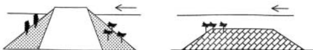
(E)緩坡度傾斜堤
