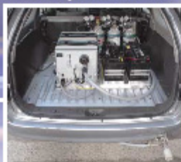
OBS-2000 system mounted in a vehicle
