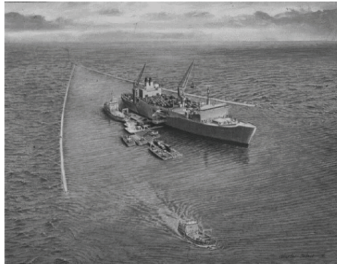
Figure 1. Rapidly Installed Breakwater System (RIBS) concept.
