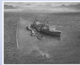
Figure 1. Rapidly Installed Breakwater System (RIBS) concept.
