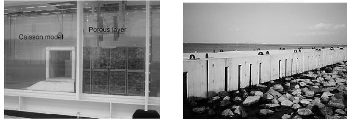
(1) Model caisson and porous layer (2) Prototype example of porous layer
