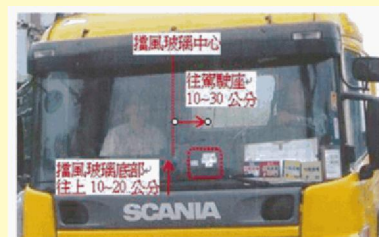
RFID Tag on the head of truck.
