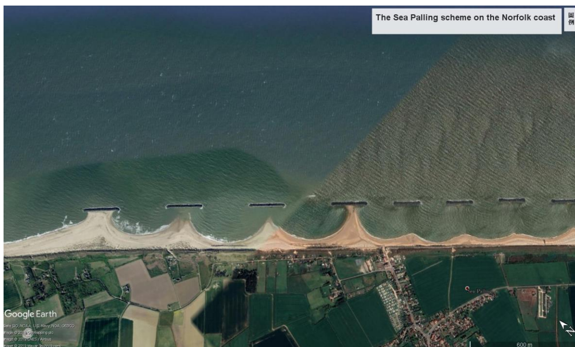
離岸堤系統_the Sea Palling on the Norfolk coast, UK_平遠大. jpg
