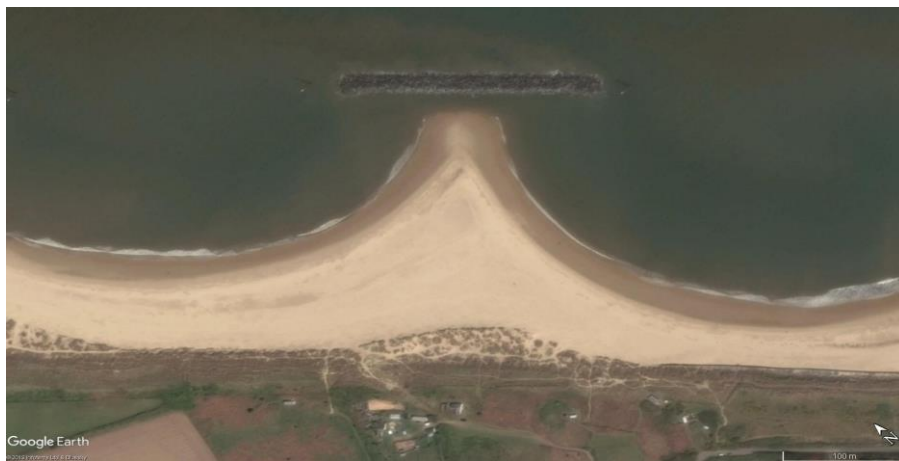
離岸堤系統_the Sea Palling on the Norfolk coast, UK_平細小_單沙舌 20150504. jpg
