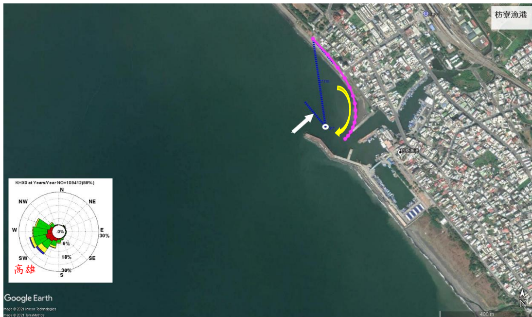
枋寮漁港_Google Earth_小_2019_10 優_岬灣海灘_玫瑰圖_卓越波向繞射點. tiff
