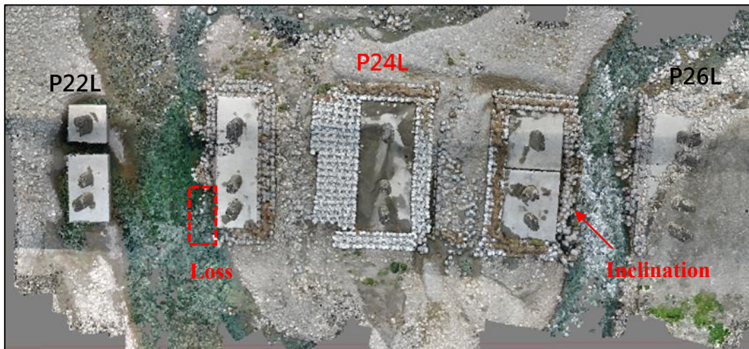
Figure 4: Comparison of the test bridge site (P24L) after typhoon flood washout with the washout situation of a nearby bridge in 2021.
