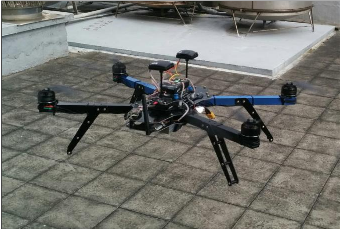
FIG. 1 Bridge inspection UVA developed and assembled by the Institute of Transportation
